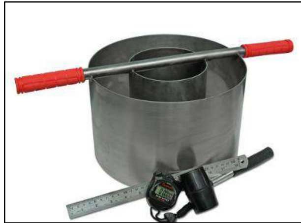
Gambar 2. 2 Alat Double Ring Infiltrometer (Sumber: Google, 2025 )
