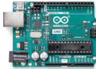
Gambar 2. 1 Mikrokontroler Arduino uno (Sumber; https://store.arduino.cc/products/arduino-uno-rev3 )
