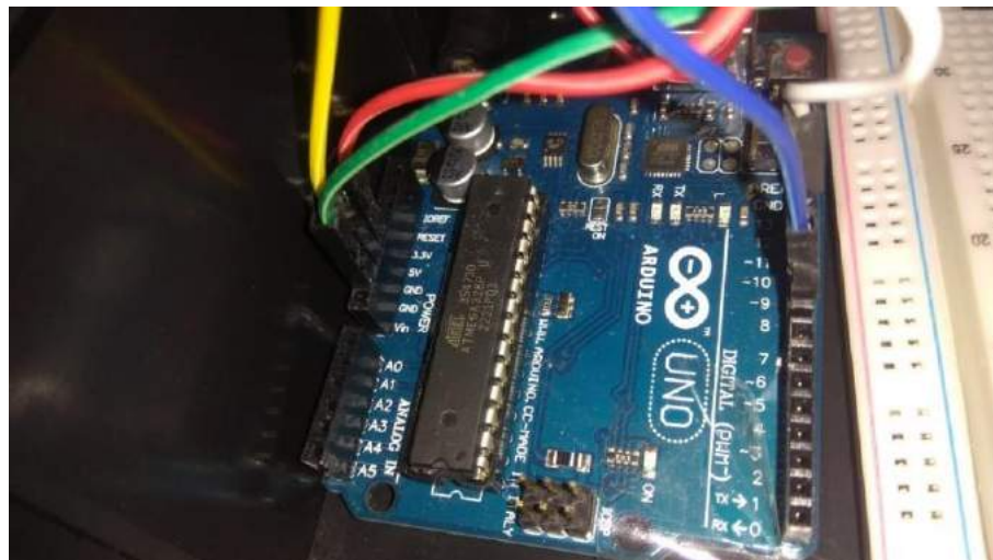
Gambar 4. 4 Pin OUT sensor ke port Arduino
