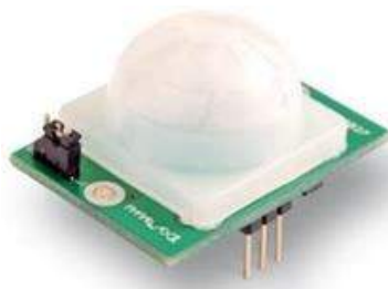
Gambar 2. 2 Sensor PIR ( Passive Infrared Receiver )
