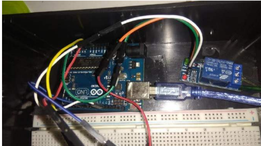
Gambar 4. 3 Pin IN Relay ke port Arduino
